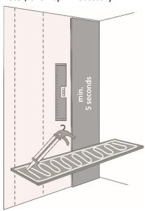
The boards can be installed with a PVC connection profile or seamlessly. For a watertight connection, a thin strip of silicone should be applied on both sides of the profile.
